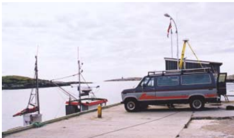
Figure 2. A Searef 200 GPS reference station was installed in the Seatex van with an L1/L2 GPS antenna on top of the van. A UHF radio transmitted DGPS corrections to the boat.
